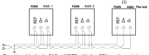
The wiring of the line for BACnet MS/TP or Modbus RTU must be carried out in accordance with applicable RS 485 standards.
